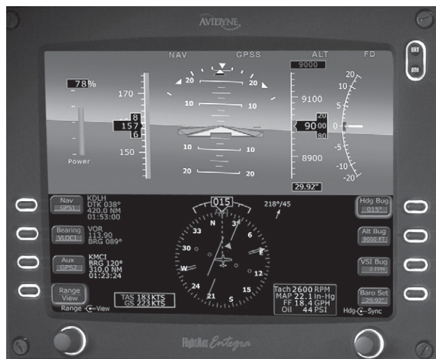
Figure 2-2. A typical primary flight display (PFD)
