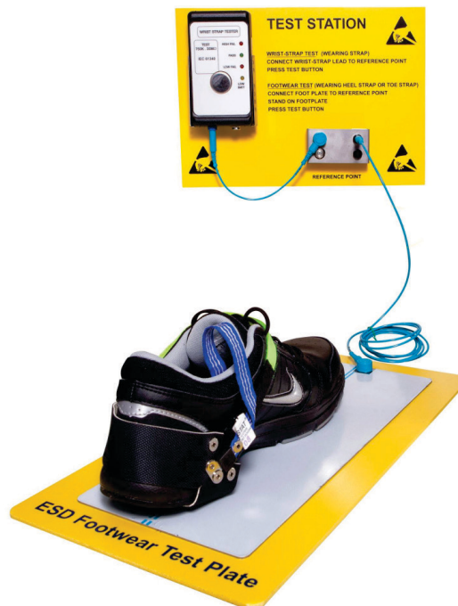
Figure 2-18. Typical grounding test station.
