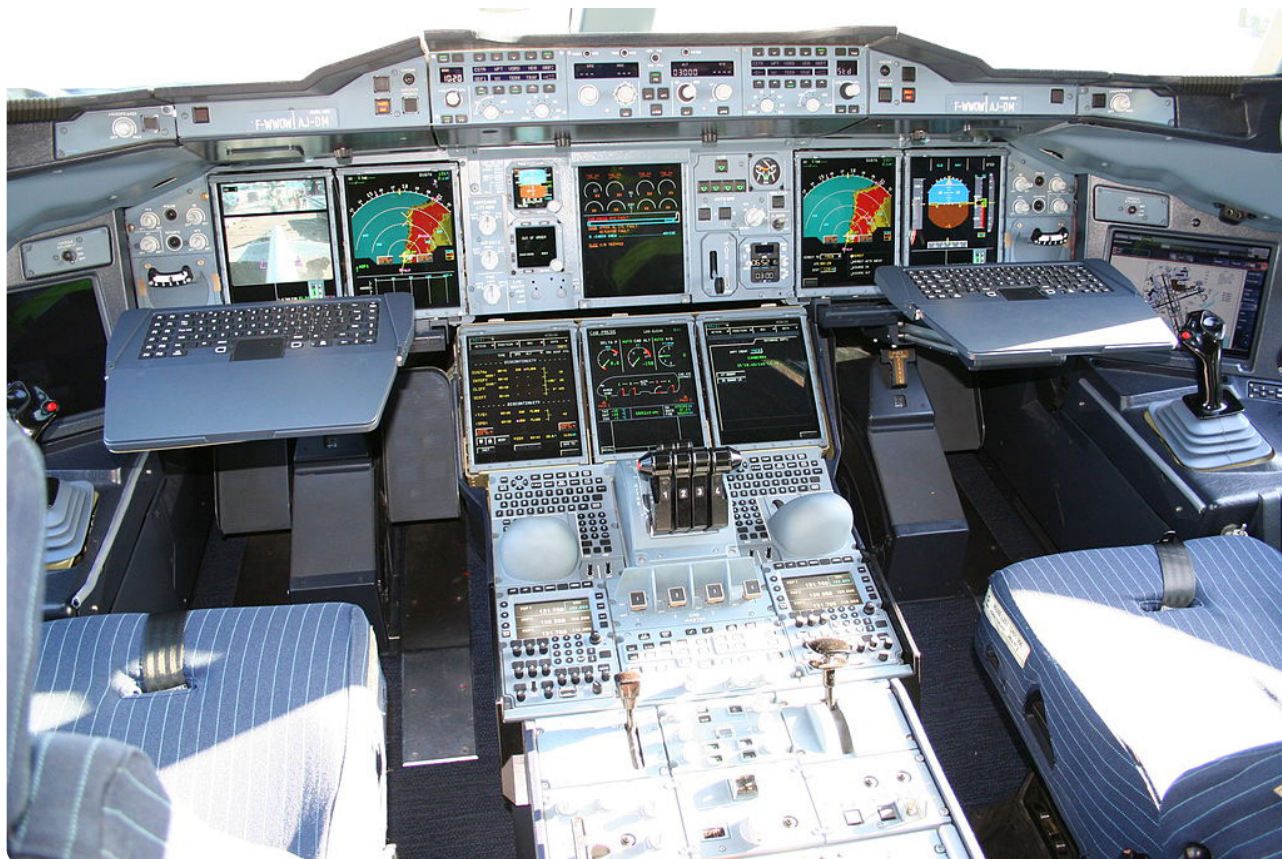
Figure 1-2. Airbus A380 EIS with 8 large LCD displays.
