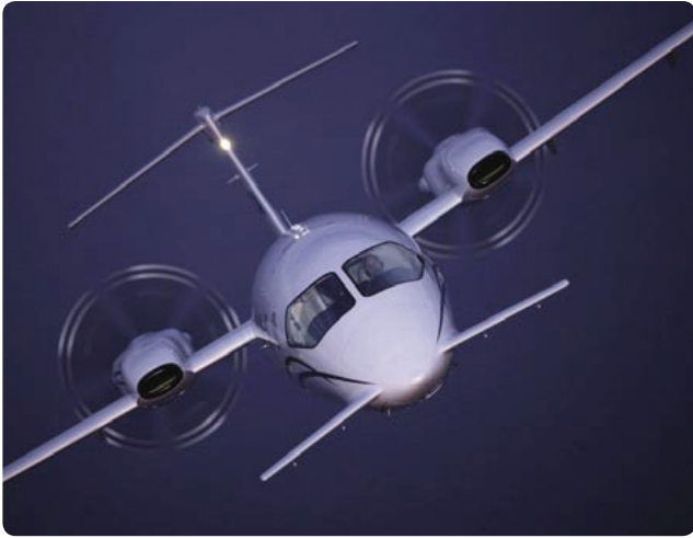
Figure 1-11. The Piaggio P180 includes a variable-sweep canard design, which provides longitudinal stability about the lateral axis.
