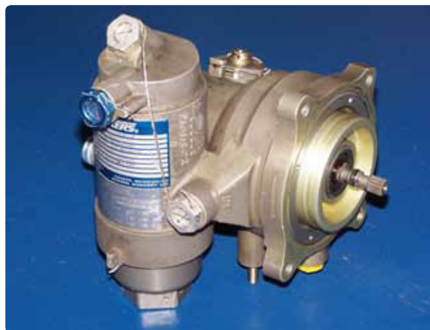
Figure 1-3. Fuel pump and filter.
