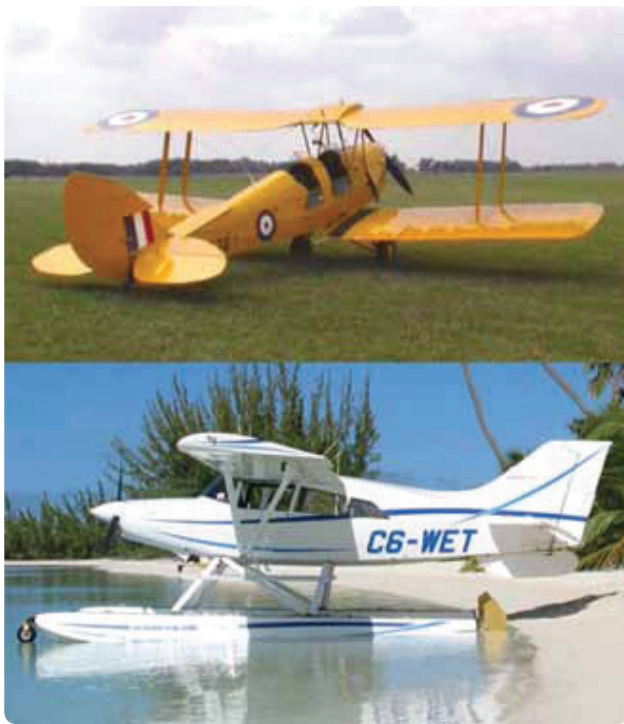
Figure 3-130. Examples of aircraft produced using fabric skin.
