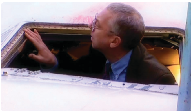
Figure 1-4. Incorrect windscreen retention bolts; (too small) led to the windshield blowout.
