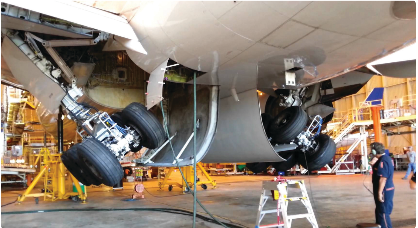
Figure 1-5. A retraction test done after the plate was fitted as opposed to prior, would have prevented damage from this accident.
